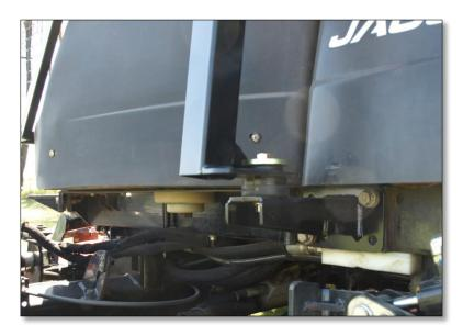
3. Take the right rear bracket and position into place where the right side of the 2-post structure was located. Use provided 1/2" x 1" hex bolts and loosely bolt the bracket into place.
