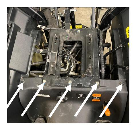
Take the underseat shield, with full upholstery cover and position it onto the seat mounting area. Slide levers through the slits in the upholstery, cutting if necessary to ensure full range of motion of controls. (old photo of shield shown)
