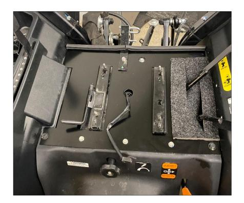
Bolt the front of the underseat shield into place with the five fasteners removed earlier.
