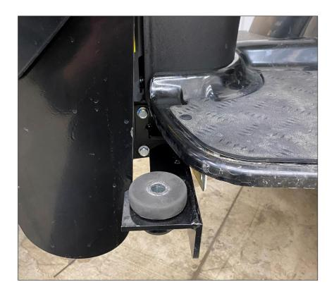
Take the right front bracket. Remove the same four fasteners at the back of the loader on the right side. Position bracket against loader, sliding carefully around the pedals and loader subframe. Fasten into place with original hardware. If no loader is present, no loader spacers will be required. DO NOT torque until later.
