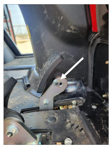
Take 12" of NDAX and install inside of lever control on right.
