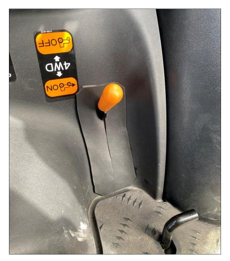
Take left lever floormat and install around pedal through platform. Peel adhesive back off and install.
