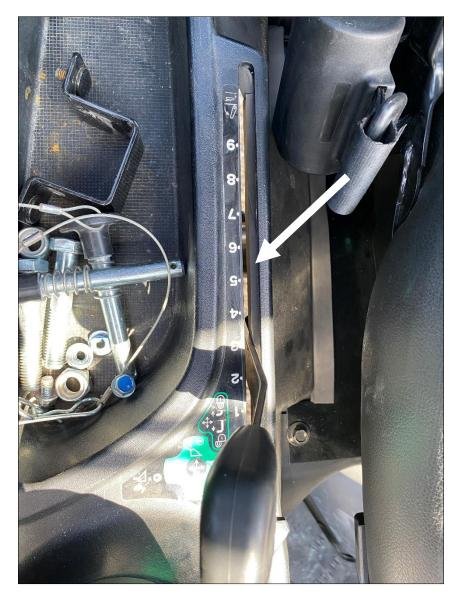
To ensure a proper weather seal, use a black silicone sealant around all small open cracks between the cab weather stripping and the tractor components.
