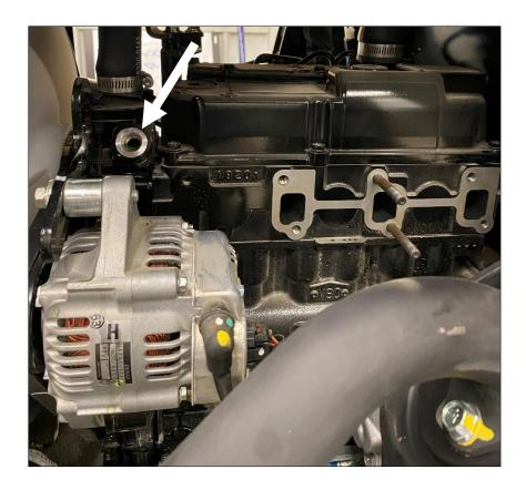
Install elbow fitting, 3/8NPT x 3/8" barb into open port on fitting just installed.
