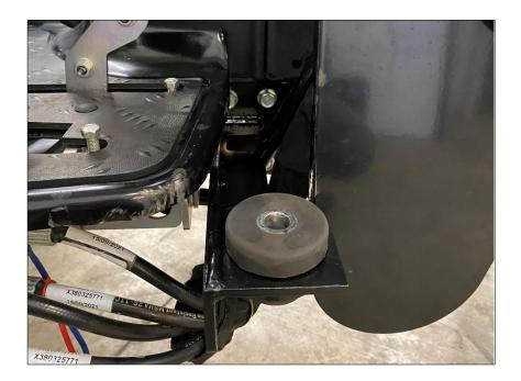
Take one of the rear brackets and position on top of the lower left 2-post ROPS, with the mounting plate facing forward. Use the provided  $\frac{1}{2}$ " x 3  $\frac{1}{2}$ " hex bolts and flange nuts to loosely attach the bracket to the 2-post. DO NOT torque until later.
