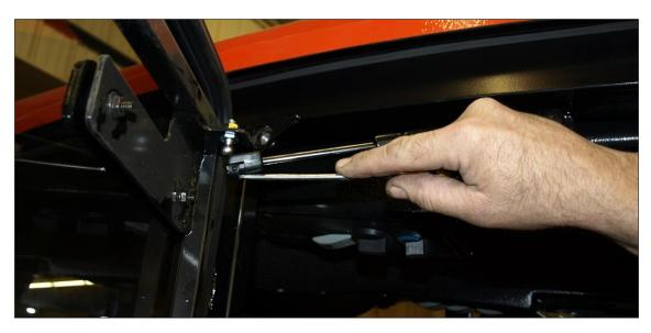
Take one of the  $\frac{1}{2}$ " x 4  $\frac{1}{2}$ " hex bolts and fasten to the weld nut located at the top rear corner of the door opening on the left side. Repeat for the right side. These are the cab lift bolts.
