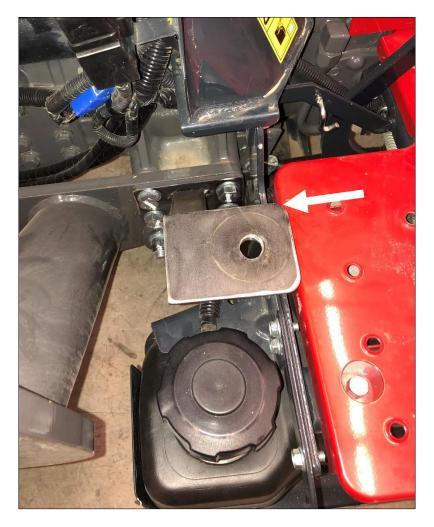
. Take the right front mounting bracket. Remove the four fasteners shown below. The hydraulic fitting shown may need to be rotated slightly to provide clearance.
