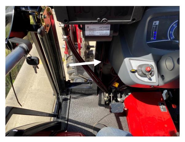
. Take the right front lower cab shield and re-install onto cab. Position on outside of the cab and fasten into place with original bolts and nuts.
