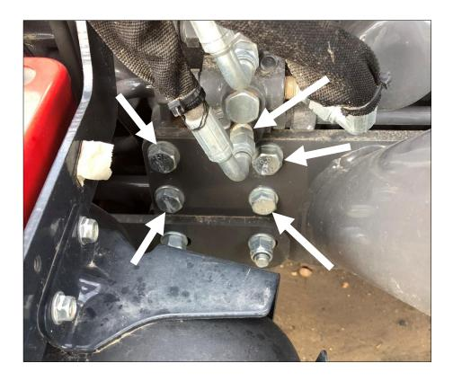
. Position the front bracket into place, re-use factory bolts and loosely fasten bracket into place.
