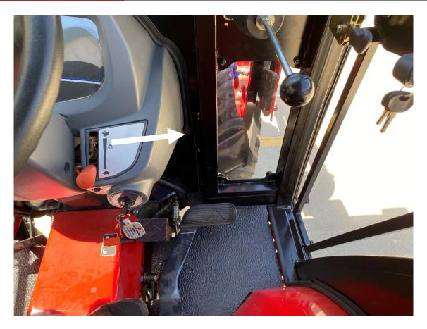
. Route the main power harness toward the engine bay from the cab A-post. Connect the black wire to the battery negative terminal. Use the provided ¼" loop, shorten wire if necessary, then solder on loop. Connect the red wire to the battery positive terminal. Use the provided ¼" loop, shorten wire if necessary, then solder on loop.
