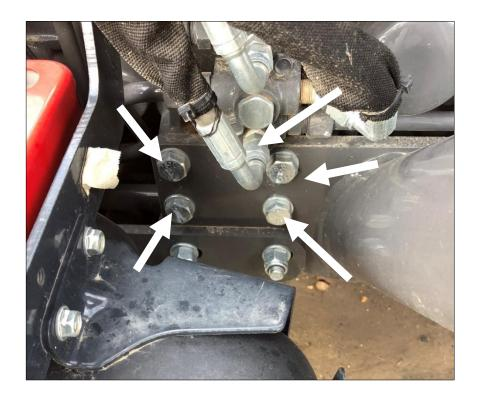
Position the front bracket into place, re-use factory bolts and loosely fasten bracket into place.
