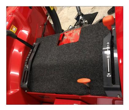
Re-install the seat mount bracket and re-connect seat harness underneath the seat plate.
