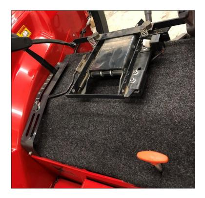
Take the left front mounting bracket. Remove the four fasteners shown below.
