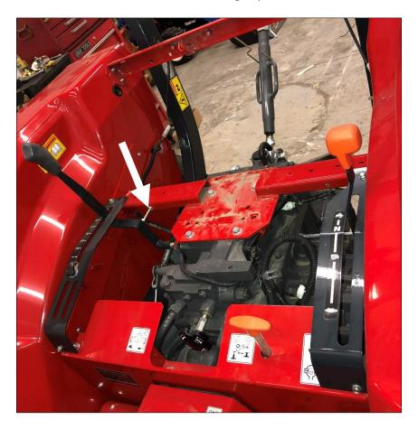
Take the under-seat shield and position it onto the tractor, between the fenders, around the seat plate.
