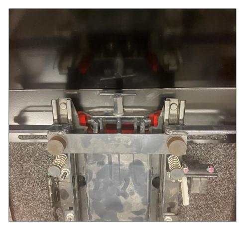
Take the clevis pin and re-install the seat onto the tractor.
