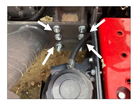
Position the left front bracket into place and using factory bolts, loosely bolt bracket into place.
