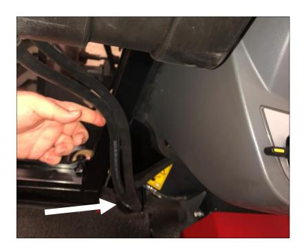
Locate the coolant bypass hose and remove.
