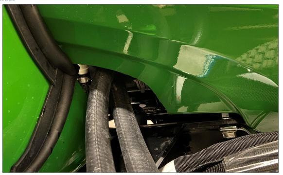
9. To ensure a better seal of all weather stripping and floor mat pieces, it is recommended that you use a black silicone seal to seal the cab parts to the tractor.
