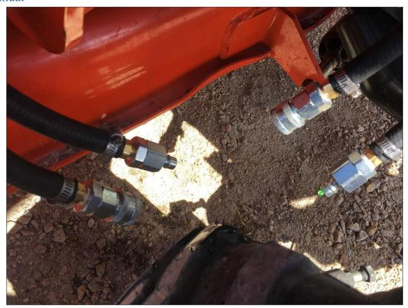
Please note, the quick-connect fittings have built-in valves to close them when they are disconnected. There should be no leakage when disconnected.
