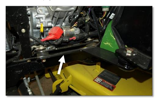
2. Repeat step 1 for the right engine mount bushings and install the front right mount bracket. Do not fully tighten until after cab is installed.
