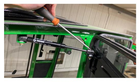
10. Take the provided cab lift bolts,  $\frac{1}{2}$  x 4 1/2" hex bolts, and install into lift weld nut that is located behind the tab at the top of the door opening.
