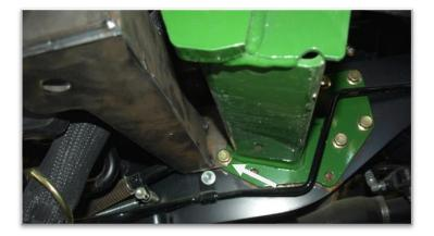
9. Remove the left and right cab doors from the cab by un-hooking the gas springs. To remove the gas shock on the left cab door, slide a flat screwdriver underneath the small clip on the end cap that must be pulled UP in order to pop the shock off of the ball stud. **The shock will release VERY easily when this is accomplished.** Lift the door assembly straight up and off of the cab, and put aside for now. Repeat for the right side.
