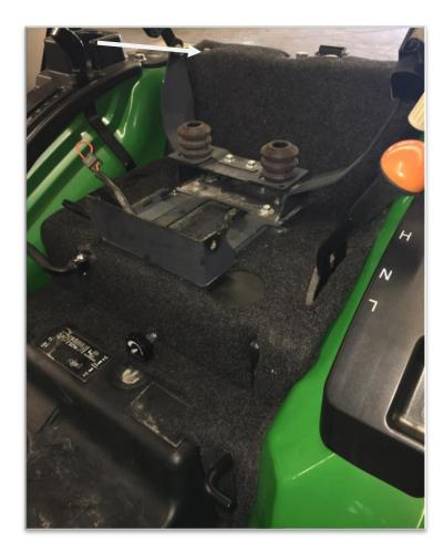
6. Re-install the control levers and end caps along with the tractor seat.
