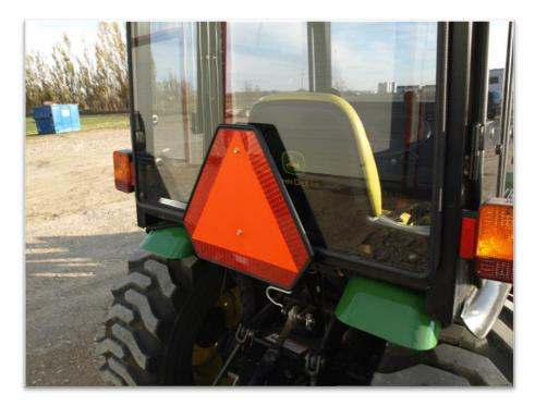
17. Take the left tractor flasher light and bolt onto the cab through the left C-post. Use the factory hardware. Route the wire harness through the centre large hole and down the post. Re-connect the wiring harness to the tractor harness. Repeat for the right flasher light.
