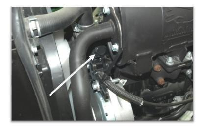
26. Locate the hoses at the left front of the cab. Route the hoses down through the holes in the lower front cab shield and into the engine bay. Avoid hot parts on the engine.
