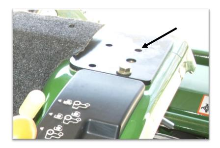
3. Remove both of the tractor grab handles to allow cab installation to be easier.
