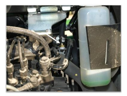
25. The suction fitting is located on the left side of the engine. Remove the plug. Use water sealant material around the threads of the fitting to prevent water leaks. Use the 16mm male x 3/8'' barb, brass o-ring and screw it into the open port. Take the remaining  $3/8NPT \times 3/8''$  barb straight fitting and install into adapter. This is the suction fitting. Muffler will need to be removed to install and the spacing is tight to the muffler.
