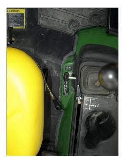
. Disconnect the seat harness plug. Remove the clevis pin that allows seat pivot, and then remove the seat from the seat track assembly. Un-bolt the seat track assembly from the tractor, the two-step process will make seat removal easier.
