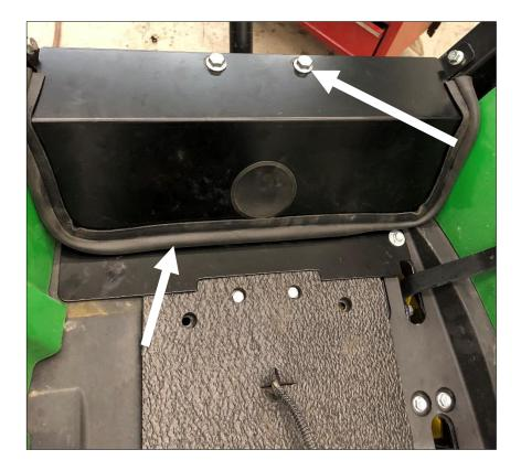
. Un-bolt upper hoop of 2-post ROPS and remove from tractor.
