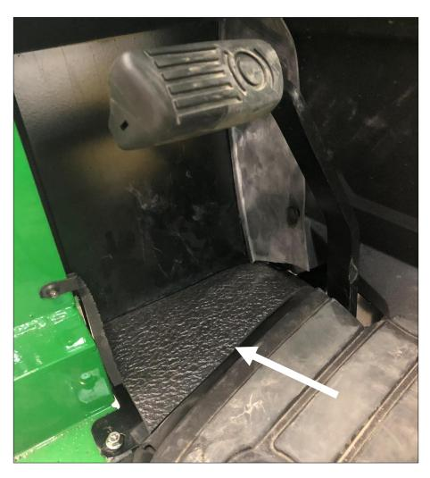
. Take the lower right pedal shield removed earlier and re-install onto cab. Ensure tight seal to tractor belly, then fasten with the  $\frac{1}{4}$ " x  $\frac{3}{4}$ " flange bolts provided.
