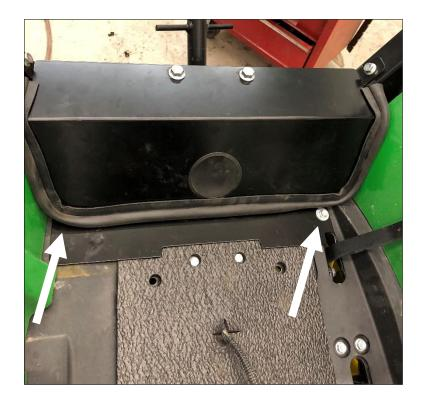
. Take the provided under seat floor-mat piece and position into cavity under the seat between the steel panel just installed and the two side plastic panels.
