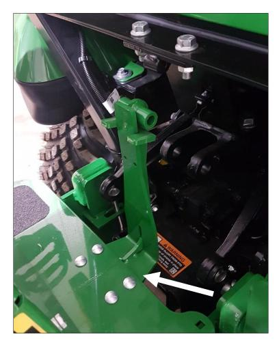
Take the provided lower backhoe seat bracket and fasten seat to the bottom plate on the hoe with the factory hardware.
