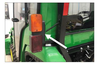
. Take the right rear flasher light removed earlier and fasten onto the plate at the right rear of the cab. Slide the harness into the cut-out area in plate, fasten to plate with provided M8 x 20 flange bolts.
