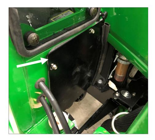
. Take the right pedal floormat pieces and position on the right pedal shield. Use provided fir tree fasteners to attach to cab shielding.
