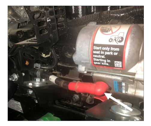
. The black wire will connect to a ground bolt on the starter, shorten wire if necessary. Use the provided ¼" loop, solder loop to black wire, and then connect to the ground bolt shown in the previous photo.
