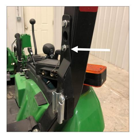
. Take the provided lift bolts,  $\frac{1}{2}$ " x 4  $\frac{1}{2}$ " hex bolts, and fasten to the cab. There are weld nuts located behind the tab at the top rear of the door opening. Install lift bolts on both sides. Use a lift strap or chain to connect both lift bolts to an overhead hoist or fork lift.
