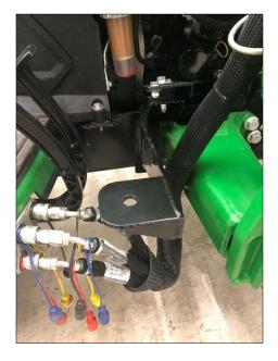
. The 5/8" fasteners can receive 205 ft-lbs of final torque. Tighten all isolators first, with the front brackets last.
