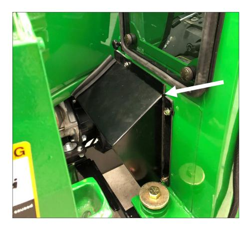
. The inner wide flap rubber needs to be fastened to the plastic shroud on tractor. Position for good seal and mark center holes. Carefully drill two 3/16" holes. Use two provided fir tree fasteners to fasten to tractor. Cut the wide flap rubber to get a good seal onto tractor.
