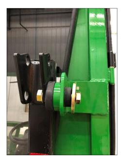
. For the front isolator fasteners, use the provided 5/8" x 3" hex bolt, ¼" heavy flat washer and flange nut in that order from above. The rear isolator uses the same order sequence. Get ALL four fasteners started before doing any final tightening.
