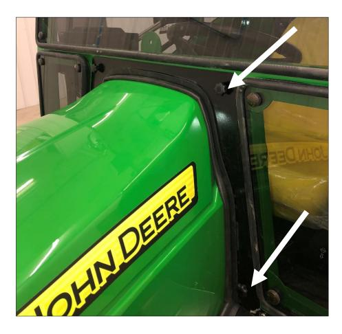
. To ensure a proper seal, use black silicone sealant around all small open cracks between the cab weather stripping and tractor components.
