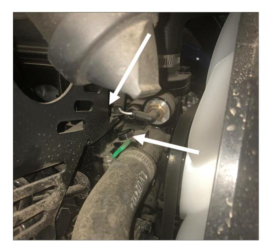
. If the finger guard is in the way remove, un-bolt and remove from the tractor. Take the provided straight 3/8NPT x 3/8" barb fitting, use silicone seal on the threads to prevent water leaks, and screw into open port.
