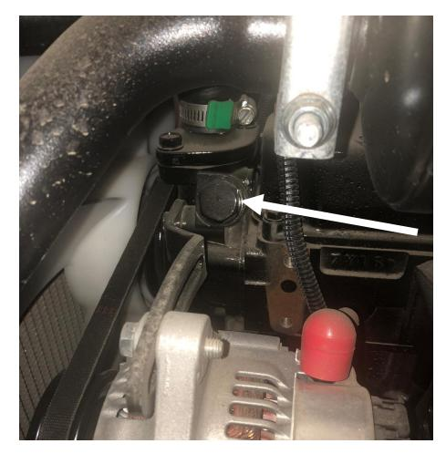
. Take the remaining straight fitting and install into the end of the metric straight adapter just installed. Ensure there is silicone on the threads of the fitting.
