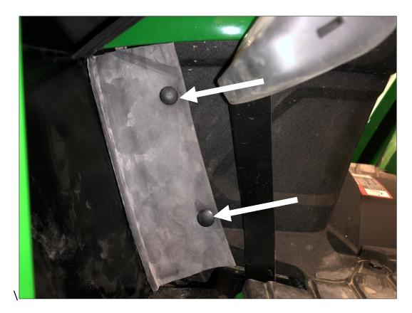
. Take the left pedal floormat and 3 fir tree fasteners. Position onto left pedal shield, aligning holes with holes in the cab sheet-metal. Install provided fir tree fasteners.
