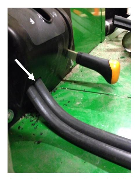
. Pull the heater hose until the hoses are sitting nice and flat on the foot platform. Place the heater hose retainer cover onto the platform to locate the ideal location. The retainer will bend easily into place while locating onto the platform. Use the provided #8 screws to retain the hose ducting. Be CAREFUL when drilling holes through platform!
