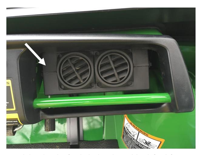
. Route the heater hoses down from the glove box and rearward along the foot platform. Notch out the area in the center black plastic console for the heater hoses to run back into the engine bay as shown below.
