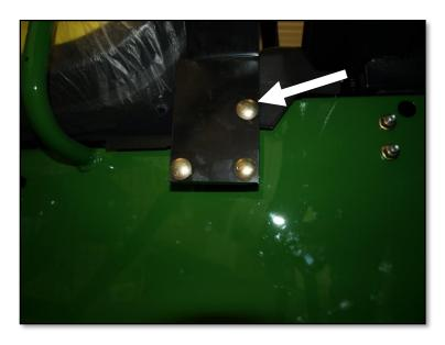
. Using the top hole in the rear bracket as a guide, drill a 5/8" hole upwards through the fender plastic.
