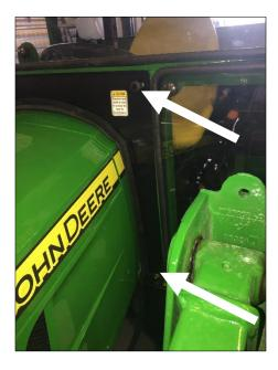
Locate the step on the tractor. Remove all four bolts fastening the step to the tractor. NOTE, the top two of the bolts need to have fasteners removed from the floorboard to allow the bolts to be completely removed.
