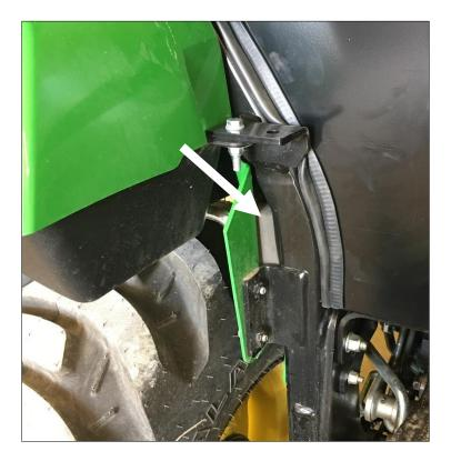
Loosen the two fasteners shown on the right side of the 2-post ROPS fastening to the fender shown below.
