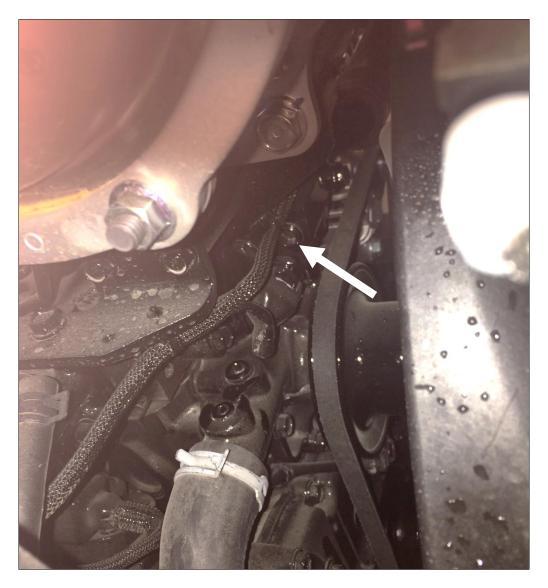
Take the provided straight  $3/8NPT \times 3/8$ " barb fitting and install Teflon tape on the threads of fitting.
