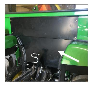
Take the left lower pedal shield and position onto cab, ensure good fit against foot platform and the bell housing of the tractor. Fasten into place with the original hardware used earlier.
