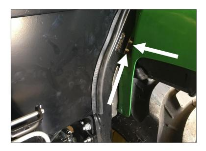
Take the remaining  $1" \times 1"$  NDAX 8" long piece and slide between the fender and the 2-post ROPS as shown below.
