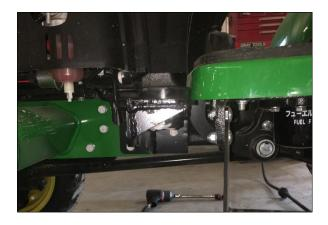
For the right front bracket, remove the rear three bolts on the loader sub-frame. One the of the fasteners retains the hydraulic mount plate.
