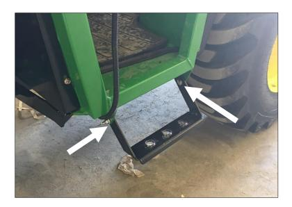
Take the left rear flasher light and route the harness through the centre large hole in the Cpost. Fasten light to the cab with factory hardware. Route harness wire down to main harness and re-connect to the tractor harness.
