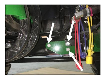
Place the right front bracket over the sub-frame and fasten into place with the factory hardware.
