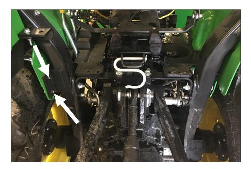
On the left side of the lower 2-post ROPS, loosen the bolts shown above.
