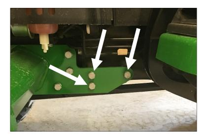
Take the left front bracket and position directly over the loader sub-frame. Use the factory hardware to fasten bracket into place.
