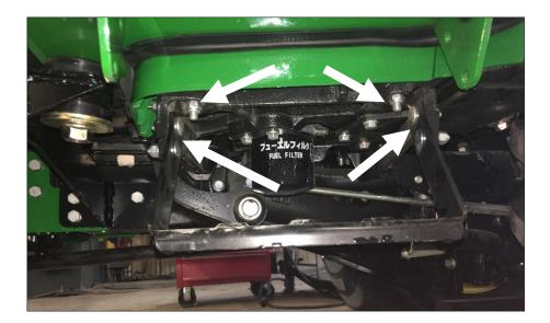
Move the step to the weld plates on the cab. Fasten step to cab with factory hardware. Reinstall floor-board bolts removed earlier.
