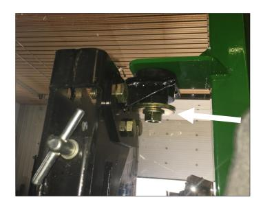
If wiper washer kits are installed, install rear brackets now with provided ¾" x 1 ½" hex bolts and flange nuts. Use caution as rear window is very close to the brackets.
