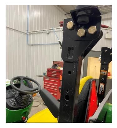
Take the right rear bracket and position against the 2-post ROPS. Using the provided  $\frac{3}{4}$ " x 1  $\frac{1}{2}$ " hex bolts and flange nuts, loosely fasten bracket into place.
