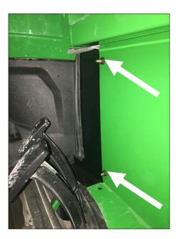
Take the hood shield and slide over the hood. Fit is tight, so it may be necessary to use soapy water on the weather seal to make it easier to install. Use the knob bolts to fasten hood shield to the cab.
