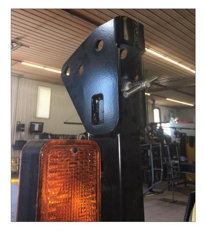
Disconnect the left 4-way flasher light harness from the tractor. Un-bolt and remove the light from the 2-post ROPS.
