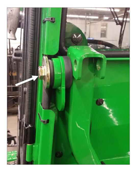
7. Use the remaining 5/8" hex bolts, flange nuts, and steel structural washer and fasten the front securely into place.
