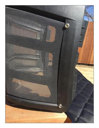
36. Drill 1/16" holes and then fasten button snap backs to the plastic shroud.
