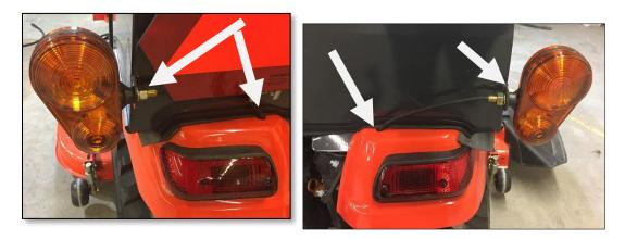
22. Take the SMV sign mount from the ROPS and attach to the rear shield of the cab, through the two holes provided with the factory hardware.
