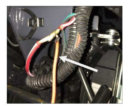
21. Take the flasher lights from the 2-post ROPS and attach to tabs at rear of cab. Route wires through hole in tab and then through the hole in the back of the fender. Re-connect the wire harnesses.
