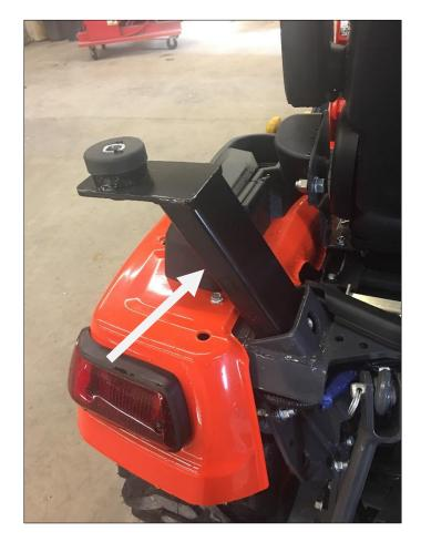
9. Take the remaining rear bracket and slide it into the open socket on the right side where the 2-post ROPS was mounted. Use the factory hardware to fasten bracket to the tractor.
