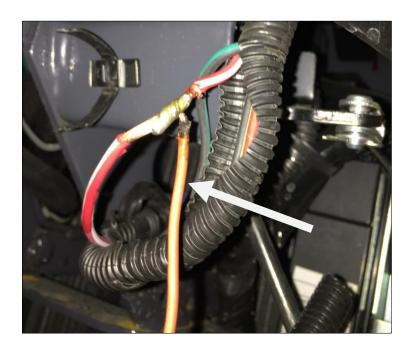
21. Take the flasher lights from the 2-post ROPS and attach to tabs at rear of cab. Route wires through hole in tab and then through the hole in the back of the fender. Re-connect the wire harnesses.
