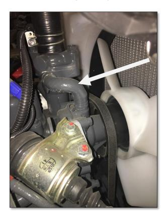
28. Route 3/8" ID hoses that are connected to heater, and go through the holes in the lower cab shielding into the engine bay. Connect the hoses to the fittings with provided HS-6 hose clamps.
