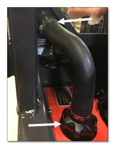
25. Two 1" holes need to be drilled into the foot platform on the right side. Install the two 1" grommets, then run the heater hose through those holes down and towards the front of the tractor.
