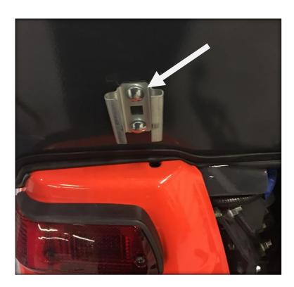
23. Take the SMV mount plate and apply bend to part that fits into sign mount. Adjust until such time that the SMV sign sits fairly straight when installed onto cab.
