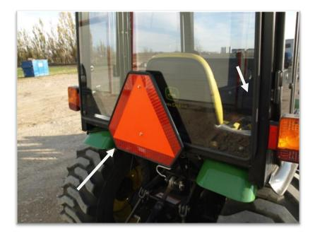
17. Take the left tractor flasher light and bolt onto the cab through the right C-post. Use the factory hardware. Route the wire harness through the centre large hole and down the post. Re-connect the wiring harness to the tractor harness. Repeat for the right tractor flasher light.
