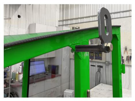
11. Attach a lift strap or chain to the lift brackets, and using a hoist or forklift, prepare to lift cab off of the shipping pallet. Un-bolt rear shipping bracket from cab, and lift cab. Position the cab over the tractor.
