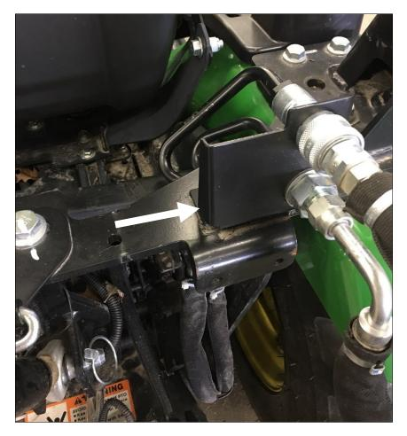
. Loosen all of the hydraulic fittings so that they can take the assembly and slide the entire assembly underneath the rear crossmember. Be VERY careful to ensure that the 3-point will not contact the hoses when lifting.
