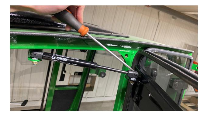
10. Take the provided cab lift brackets and  $\frac{1}{2}$ " x 4  $\frac{1}{2}$ " hex bolts and install the lift brackets onto the cab as shown below.
