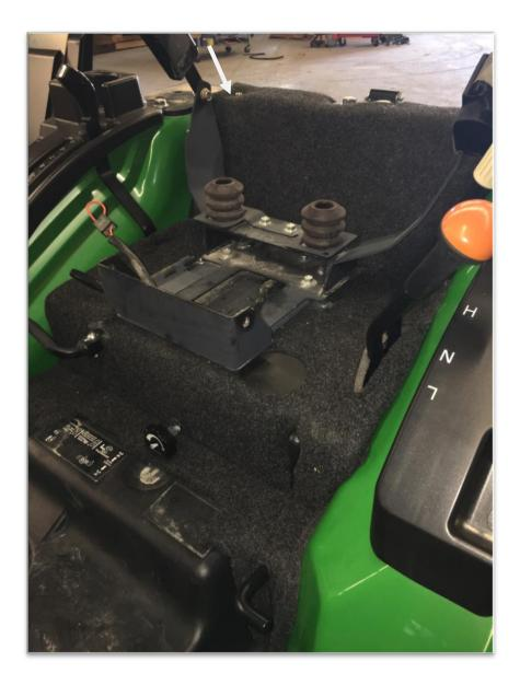
6. Re-install the control levers and end caps along with the tractor seat and seat mount.
