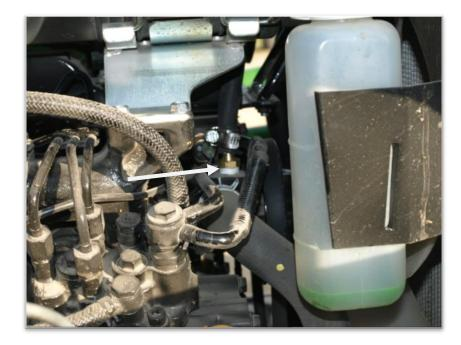
25. The suction fitting is located on the left side of the engine. Remove the plug. Use water sealant material around the threads of the fitting to prevent water leaks. Use the  $16MM \times 3/8''$  NPT straight fitting and brass o-ring and screw it into the open port. Take the remaining  $3/8NPT \times 3/8''$  barb straight fitting and install into adapter. This is the suction fitting. Muffler will need to be removed to install. NOTE, the heater hose will be close to the muffler once installed.
