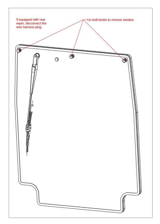
Step 2: Remove the three knob bolt fasteners at the top of the rear window to completely loosen glass from cab.
