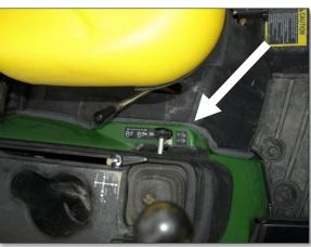
2. Un-bolt and remove the tool box bracket from the right 2-post ROPS. Save the flange bolts for re-use. Unfortunately, there is not enough room to re-mount the tool box onto the tractor.
