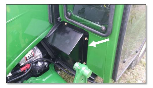
43. Re-install the right pedal shield and the remaining  $\frac{1}{4}$ " x  $\frac{3}{4}$ " flange bolts. Position the panel onto the outside front of the cab, aligning the shield with the clip nuts on the cab, and fasten into place.
