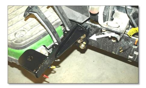
22. Take the left lower pedal shield (no notches), two  $\frac{1}{4}$ " x  $\frac{3}{4}$ " flange bolts and nuts, lift the front of the operator platform floor-mat up slightly, then tuck pedal shield underneath platform floor-mat. Use the provided flange bolts to fasten shield onto left front bracket.
