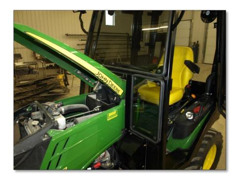
49. To ensure a proper seal, use a black silicone sealant around all small open cracks between the cab weather stripping and tractor components.
