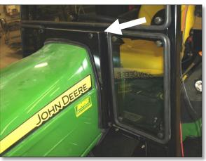
42. Re-install the left pedal shield, and three  $\frac{1}{2}$ " x  $\frac{3}{4}$ " flange bolts. Position the panel onto the outside front of the cab, aligning the shield with the clip nuts on the cab. Fasten into place.
