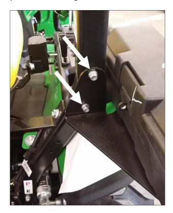
3. Un-bolt the left flasher light bracket from the 2-post ROPS (U-bolt and flange bolt).
