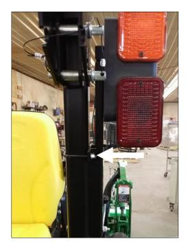
9. Take the flasher light and fasten it directly to the 2-post ROPS through the original factory holes in the 2-post. Use the M8 x 65 mm flange bolts from the tool box mount bracket.
