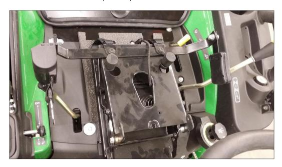
15. Remove the two fasteners in the rear cross-member between the lower 2-post ROPS members. Take the provided lower rear shield and put on top of the cross-member so that the shield goes down and forward. Fasten into place with the fasteners removed earlier.
