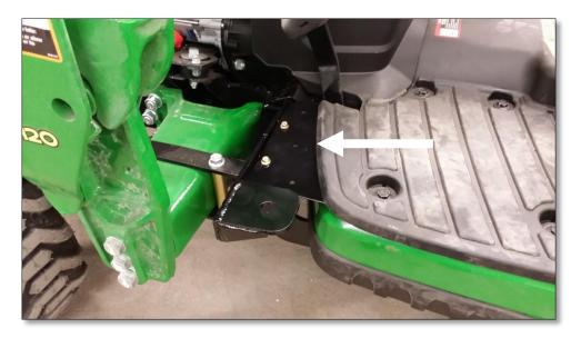
23. Take the right lower pedal shield (two notches), two  $\frac{1}{4}$ " x  $\frac{3}{4}$ " flange bolts and nuts, and lift the front of the operator platform floor-mat up slightly, then tuck pedal shield underneath platform floor-mat. Use the provided flange bolts to fasten shield onto right front bracket.
