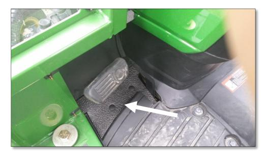
47. Take the right pedal floor-mat provided and position overtop the lower shield installed earlier and underneath the tractor factory floor-mat. Ensure the throttle pedals have full range of motion, notching if necessary. Use provided fir tree fasteners to fasten to lower pedal shield installed earlier.
