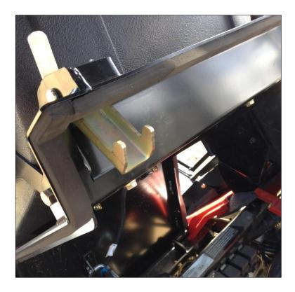
7. Take the rear cab bracket and slide into position where 2-post ROPS was mounted, with shielding on bracket sealing onto sprayer. Re-use factory hardware, and bolt into place.
