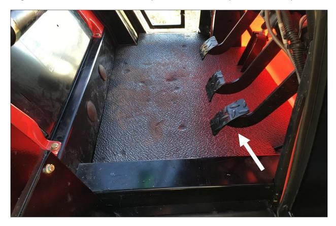
18. Take the 5" x 5" piece of floormat along with the two fir tree fasteners and position underneath the right console of the sprayer. Drill two  $\frac{1}{4}$ " holes and retain floormat to machine.
