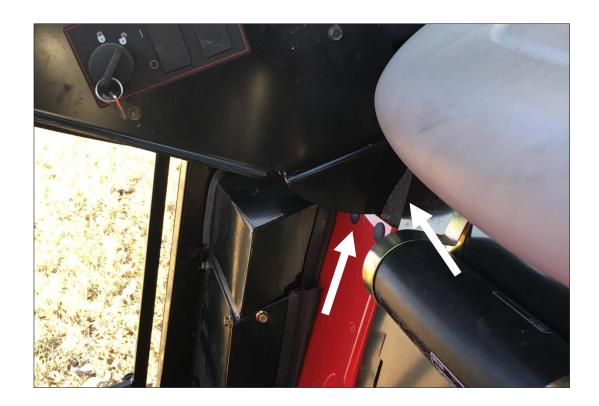
19. Take the shield removed earlier and re-fasten to the cab with the original fasteners.
