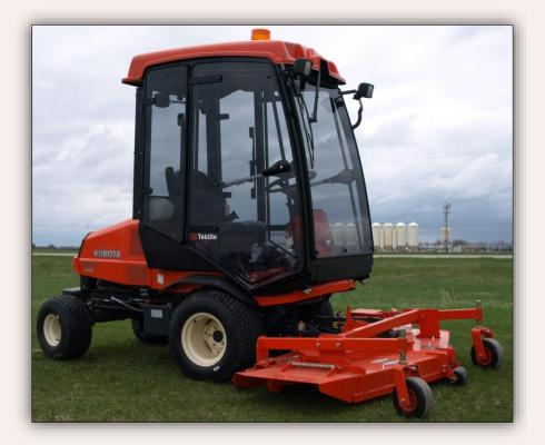
Kubota Fx80 Series Cab This ROPS cab is designed and built to fit the Kubota F2880, F3080, and F3680. Designed and Built by: Tektite Manufacturing Inc: 427 Buffalo Street P.O. Box 639 Winkler, MB R6W 4A8 Canada PH: 204-331-3463 Fax: 204-331-4159 sales@tektite.ca www.tektite.ca
