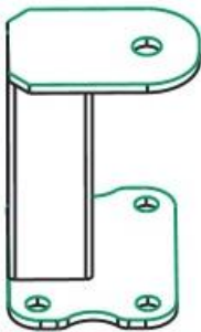
Rear Brackets Top Plate 4 9/16" in length
