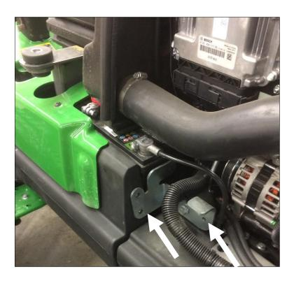
Remove the battery from the machine.
