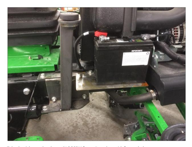
Take the right rear bracket and LOOSELY fasten into place with factory bolts.
