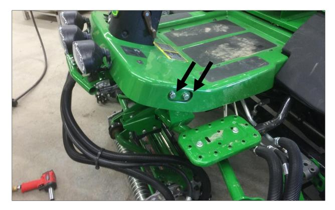
Take the left front bracket and squeeze in between the platform and steel plate inside of platform. Use factory hardware and bold bracket into place. NOTE: steel sub-frame will want to fall down and out once fasteners are removed. (Right side shown below)
