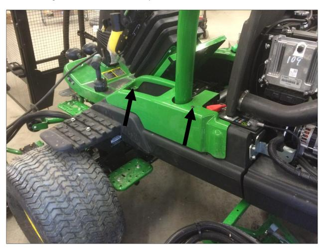
Remove the fasteners through the top of the black left side pod.
