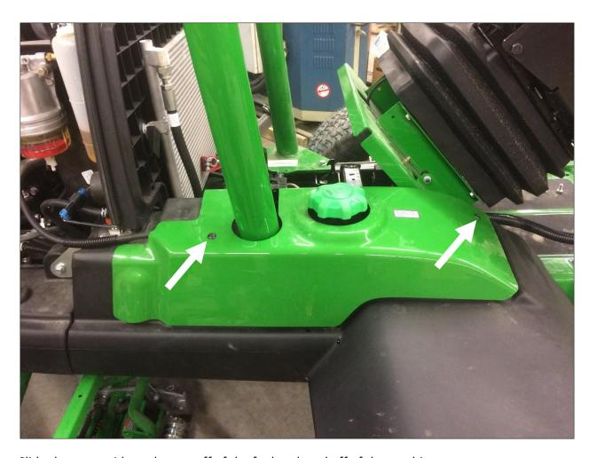
Slide the green side pod cover off of the fuel tank and off of the machine.
