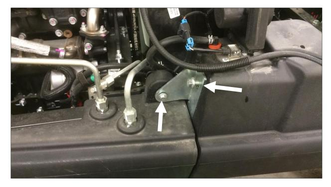
Disconnect the sensor and the fuel hose line at the front and back of the tank. This will later allow COMPLETE removal of the fuel tank from the mower chassis.
