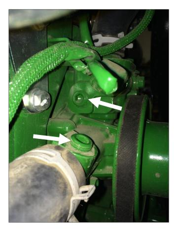
33. Take one of the 3/8NPT x 3/8" barb fittings and install into the open port on the thermostat housing. Use a water sealant around the threads to prevent any water leaks.
