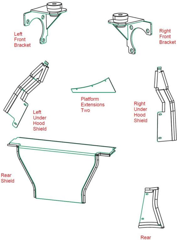
Rear Shield L&R NOTE: All references to left and right, front to back are from the perspective of sitting on the seat facing forward on the tractor.
