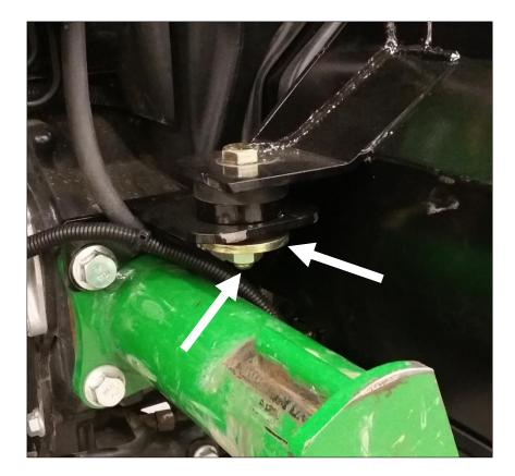
19. For the rear mounts, use  $5/8" \times 5"$  hex bolts, heavy flat washers, and flange nuts. The flat washer and nut go on the inside of the cab. The middle fastener hole, front to back is used on the 2-post mount.
