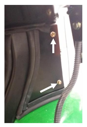
29. Take the left front under-hood shield and slide around brake pedals and up against the cab. Ensure good fit, then fasten into place with 1/4" x 1/2" flange bolts.
