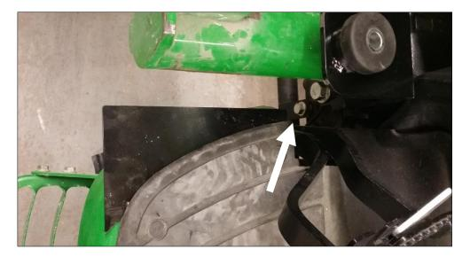
11. Take the remaining front platform extension shield and  $#8 \times 1"$  screws. Pull back the front right corner of the operator platform floormat and position the shield onto steel platform. Align inside with the edge of the cut-out in the platform. Shield should follow platform curve. Use screws provided to fasten the shield to the platform.
