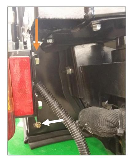
28. Take the right rear side fender shield and position against the 2-post ROPS, right side cab panel, and the rear shield. Ensure a good seal to 2-post ROPS, then fasten to cab with two of the provided  $1/4" \times 1/2"$  flange bolts. NOTE: This joint needs to be sealed with black silicone.
