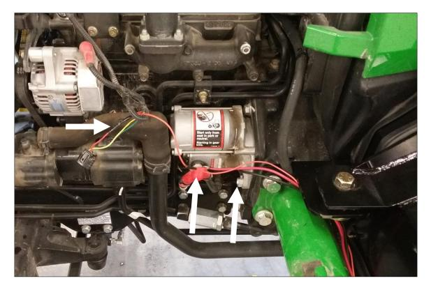
23. Main power (10GA red wire) is to be connected to the starter, with the provided 1/4" loop connector. If necessary, shorten the wire, then install onto wire and solder the connection.
