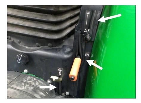
8. Take the 4 1/4" long 180 degree bulb seal and position it onto the left side of the plastic shroud of the front wheel assist lever.
