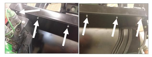
27. Take the left rear side fender shield and position against the 2-post ROPS, left side cab panel, and the rear shield. Ensure a good seal to 2-post ROPS, then fasten to cab with two of the provided  $1/4" \times 1/2"$  flange bolts. NOTE: This joint needs to be sealed with black silicone.
