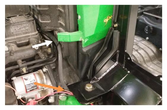
36. Take the hose coming out of the right A-post, and route into the engine bay, along the firewall, and up and over the air intake towards the open fitting on the water pump. Shorten hose if necessary, then connect to fitting. Use the provided HS-6 hose clamp to tighten hose.
