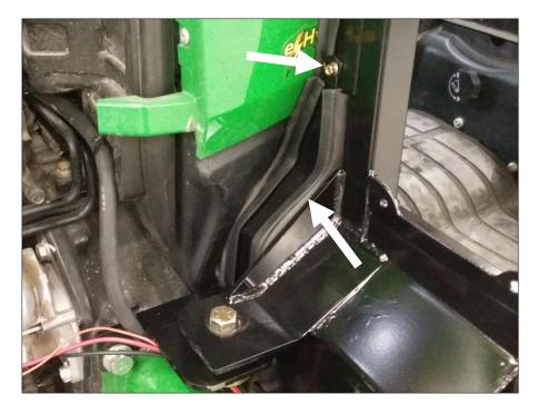
30. Take the right front under-hood shield and slide into position up against the cab and the tractor. Ensure good fit, then fasten into place with  $1/4" \times 1/2"$  flange bolts.
