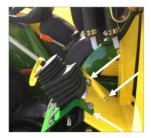
. Locate the wiring harness coming out of the front left A-post of the cab. Route towards the starter on the left side of the engine.
