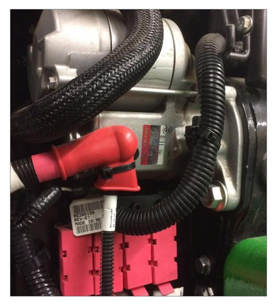
. Connect the black wire to a ground bolt. Use the provided loop connector, shorten wire if necessary, crimp on connector then fasten to ground bolt on the tractor.
