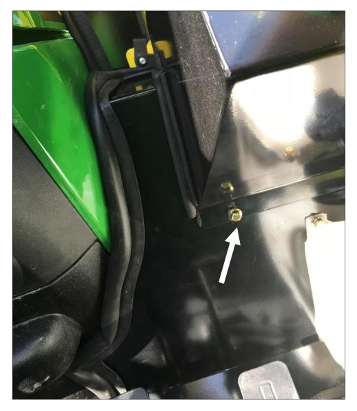
. Take the valve control cover and position around the valve and against the cab. Fasten to the lower right front shield installed earlier and the loader valve mount plate on the cab.
