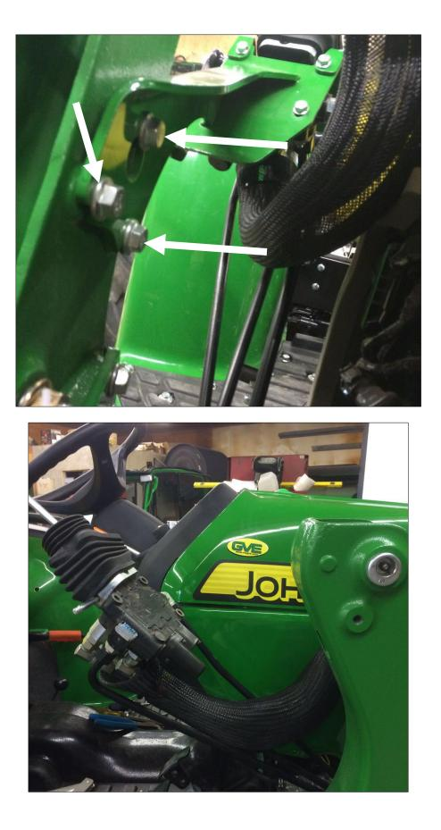
. Un-bolt the rear two fasteners from the loader sub-frame. Take the provided left front bracket and two ¼" washer spacers. Position the spacers behind the bracket and then fasten to the tractor through the rear holes of the loader sub-frame with factory bolts.
