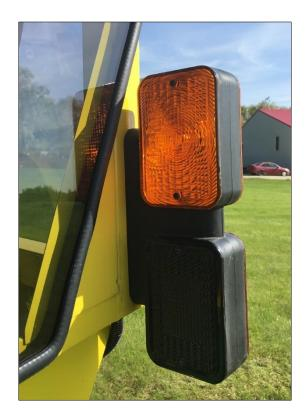
. Take the right flasher light removed earlier and route the harness through the large hole in the C-post. Fasten to the cab with the factory bolts and nuts.
