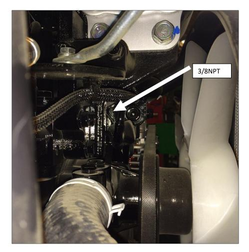
. Take the provided  $3/8NPT \times 3/8''$  barb straight fitting, use a silicone sealant on the threads to prevent water leaks, and install one fitting into 3/8NPT open port on the engine.
