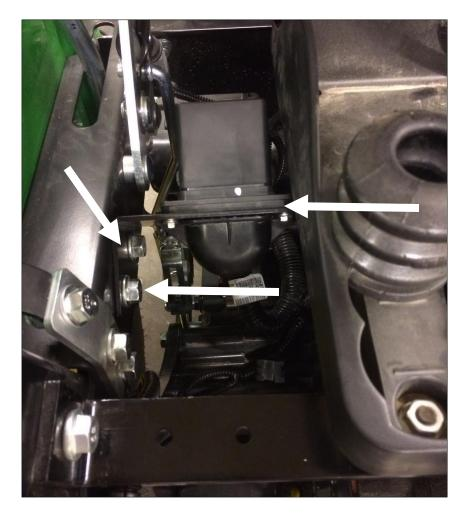
. Take the upholstered under seat shield provided and position it on the seat platform area. Take fuse block and install under rear cab shield with factory fasteners and one of the provided  $\frac{1}{4}$ " x  $\frac{3}{4}$ " flange bolts.
