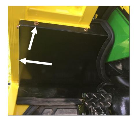
. Re-install the right front panel on the cab.
