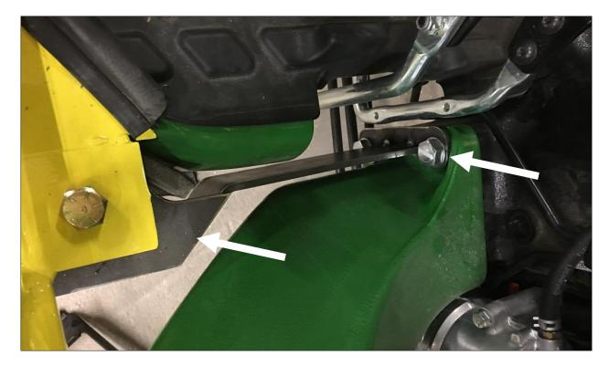
NOTE: For the right front bracket, the pedals are VERY tight to the bracket plate. It may be necessary to adjust the linkages to prevent interference to the bracket.
