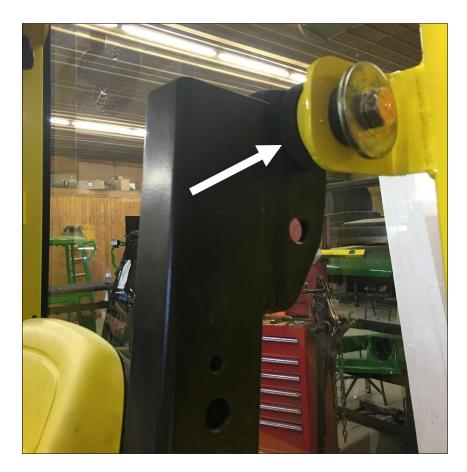
. Use the provided 5/8" x 5" hex bolt, heavy ¼" flat washer, and 5/8" flange nut for the rear isolator position, NOTE alignment of bolt in photo above. Start bolts only at this point, do not tighten until all fasteners are started.
