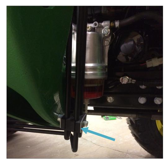
. Un-bolt the three fasteners shown that fasten the valve to the support bracket.
