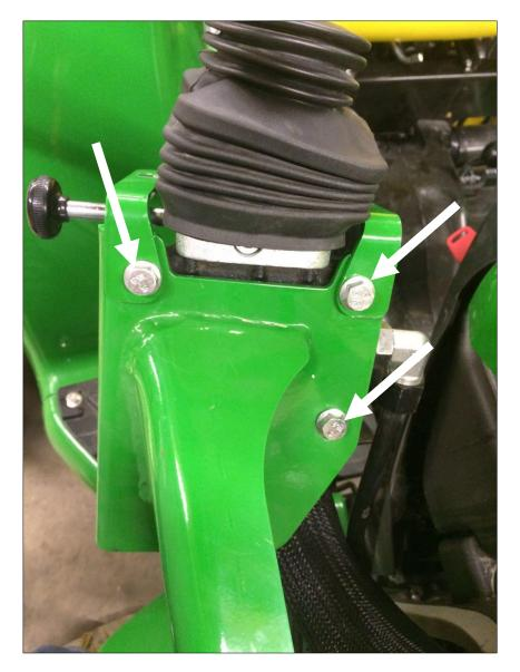
. Un-bolt the three fasteners that attach the loader valve bracket to the loader sub-frame shown on next page. Let the valve assembly hang as is.
