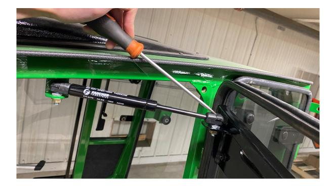
. Un-hook the gas shock on the right cab door using the same procedure. Lift the door assembly straight up and off of the cab and put aside for now.
