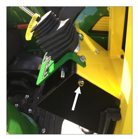
. Remove the SMV sign from the tractor. Fasten to the rear shield of the cab with the provided  $\frac{1}{2}$ " x  $\frac{1}{2}$ " flange bolts and nuts.
