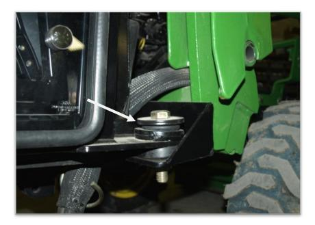
14. Use the same alignment procedure for the front bracket isolators (3" bolts). Once all 4 bolts have been started, you can apply final torques. For the ROPS isolators, 200-ft-lbs is required. For the M12 bell housing fasteners, use 97 ft-lbs.
