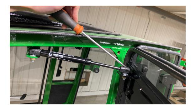
10. Take the provided cab lift brackets and  $\frac{1}{2}$ " x 4  $\frac{1}{2}$ " hex bolts and install the lift brackets onto the cab as shown below.
