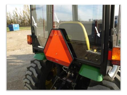
17. Take the right tractor flasher light and bolt onto the cab through the right C-post. Use the factory hardware. Route the wire harness through the centre large hole and down the post. Re-connect the wiring harness to the tractor harness. Repeat for the left tractor flasher light.
