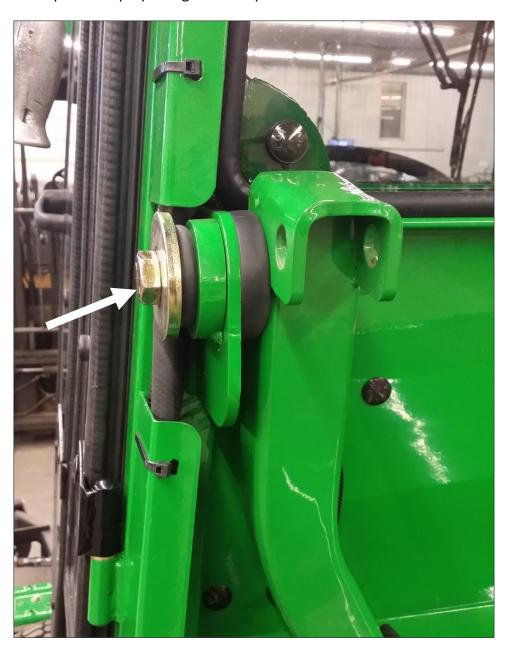
16. Use the remaining 5/8" hex bolts, flange nuts, and steel structural washer and fasten the front into place.
