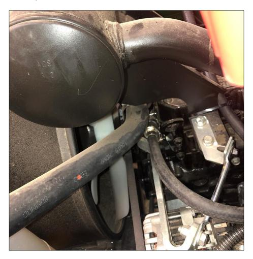
24. Locate the lower radiator hose on the left side of the engine. Mark and cut the radiator hose directly in front of the part number. Take the provided 1 1/8" radiator hose splicer (for **1550 ONLY**) and install on the radiator hose with the HS-24 hose clamps. Take the 3/8NPT x 3/8" barb straight fitting and screw it into the splicer. This is the suction fitting. The **1570 & 1580** use the 1 3/8" radiator splicer.
