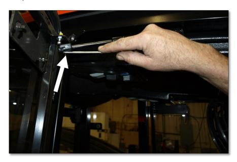
11. Take one cab lift bracket along with one ½" x 4 ½" hex bolt and bolt the lift bracket to the mounting tab that it is at the back top corner of the door opening. Repeat for the opposite side.
