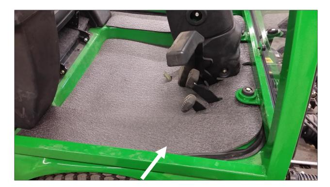
18. Locate the main electrical harness at the back left corner of the cab and route into the engine compartment along with the heater hoses.
