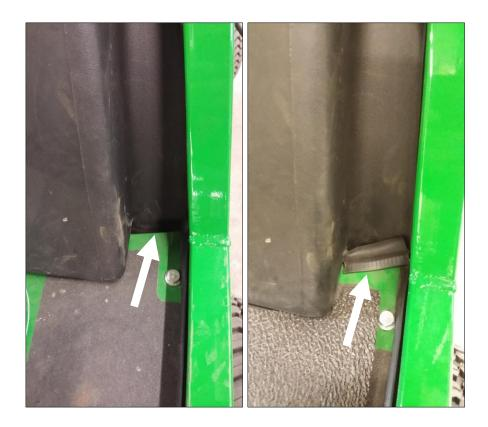
9. Take the other 3" long pieces of 180 degree bulb seal and install on the right side tank position.
